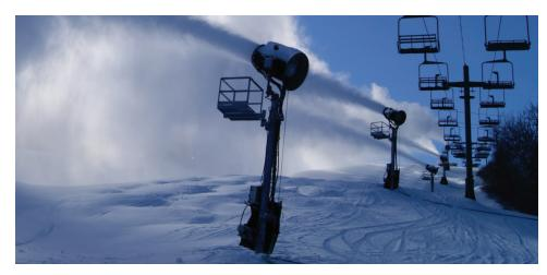
We were able to buy efficient snow guns, increase the size of the pond, go from pumping 1,800 gallons per minute to 3,300 gallons per minute, and we're using less energy.
